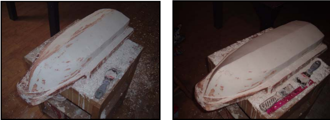
Figure 7: Detailing the plaster cast of the hull
