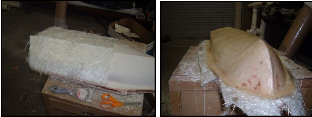
Figure 8: Dry Fiberglass and Fiberglass with Resin Hardener
