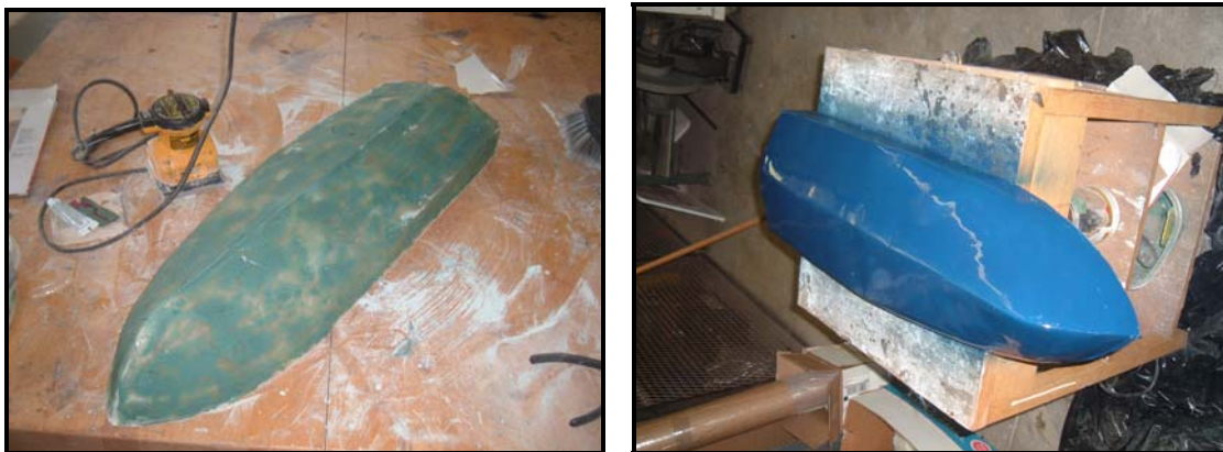
Figure 9: Fiberglass With Sanded “Bondo” and Hull With One Coat of Paint
