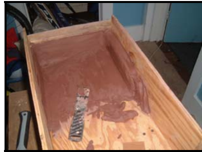
Figure 5: Shaping the clay cast of the hull
