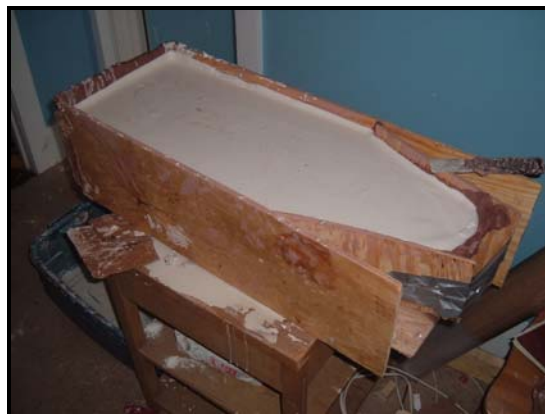
Figure 6: Plaster Cast Poured Into The Clay Mold
