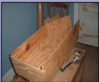
1. Building a molding frame and shaping clay to hull specs
