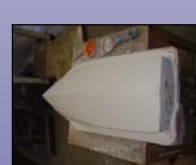
2. Casting the clay hull with molding plaster
