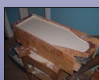
2. Casting the clay hull with molding plaster
