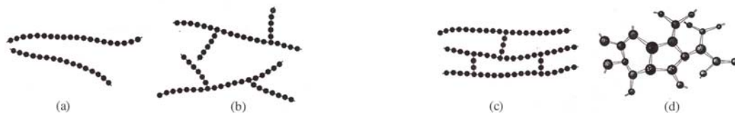
Figure 2: Schematic illustrations of (a) linear, (b) branched, (c) crosslinked, and (d) network 3-D molecular structures. The circles indicate individual mer units.
